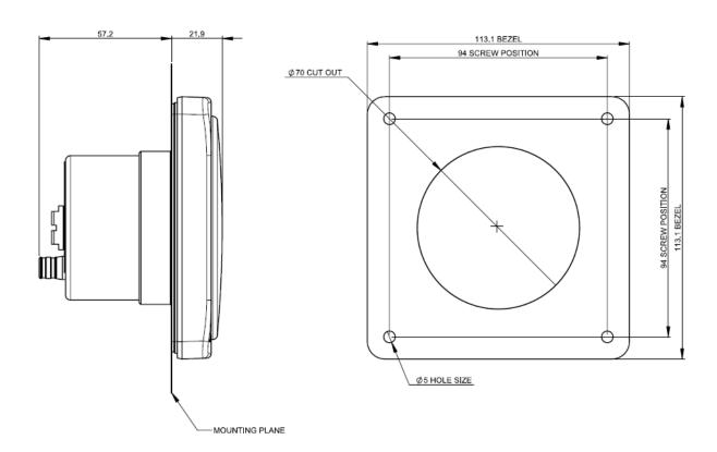
**NOTE:** The fastening hole locations of a B&G H2000 Analogue display vary and may not exactly match the A+T Analogue display. They may require re-drilling to fit.
