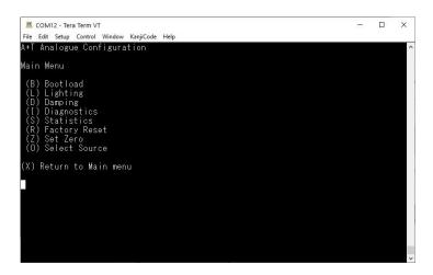
The system menu is operated by keyboard keys. For example to adjust the lighting levels press L to enter the lighting menu, or to set the CANbus (N2k) data source, press O.
