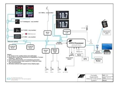
Typical Superyacht ATP2 Ethernet Instrument Configuration
